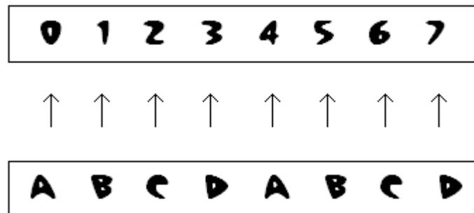
Essentially these two streams (after further ciphering) are combined to produce a *keystream* which will ultimately be combined with the plaintext input, via an exclusive or [XOR] operation - producing the cipher text. This combined cipher is known as the *Vernam Cipher*.
